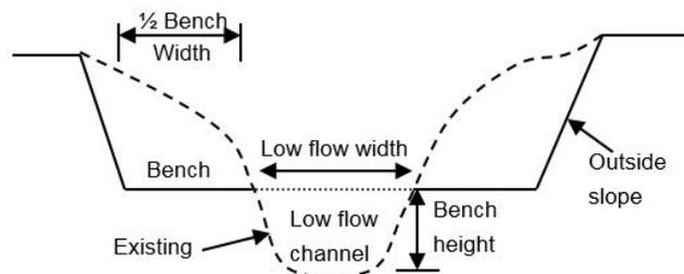
**Figure 1.** Typical Two-sided Two-stage Ditch
