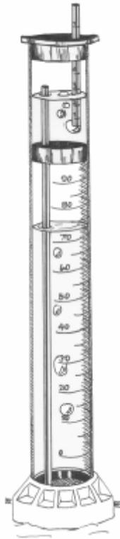
**Figure 3.2: Illustration of the Minidisk infiltrrometer (Source: Decagon Devices, 2005).**
