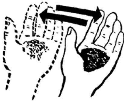
Dilatancy test: Shaking wet soil
