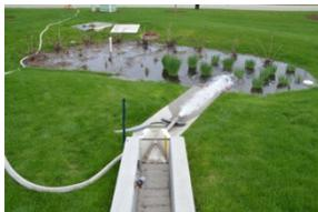
Figure9. Fire Hose flushing test at Cell 3.
