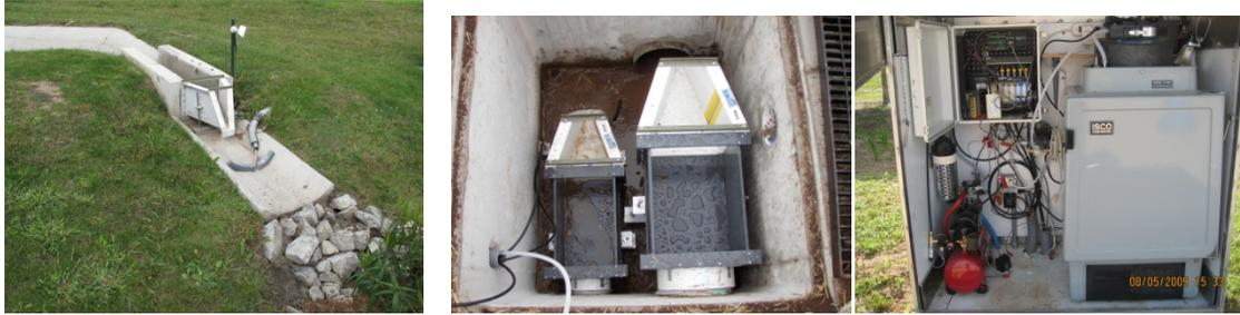
Figure 5. The inlet, outlet, and automatic monitoring equipment installed at each site.
